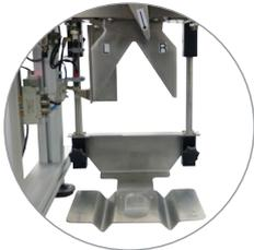
The dual outlet can be adjusted for bags of different sizes, making it a flexible solution, ideal for field trial preparation where thousands of bags need to be filled within a short time.
